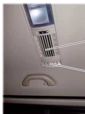
Nozzles in headlining - for air-conditioning the compartment air
